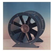
For Duct Mounted applications moving clean or contaminated air supply and extraction. They can be fitted with Standard or Atex rated motors with single or 3 phase supply. Fan casings can also be fabricated in 304 and 316 Stainless Steel.
